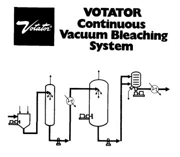
For the continuous bleaching of edible fats and oils • Excellent color reduction and soap removal • Low clay dosage. Low oil retention • Effective deaeration and dehydration. Effective oil-clay contact • Efficient utility usage. Minimum operator attention • Automatic control of process variables.
